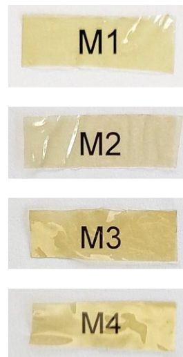
Figure S 11: Optical images of the blend membranes M1, M2, M3 and M4 highlighting their transparency, homogeneity and absence of precipitates.
