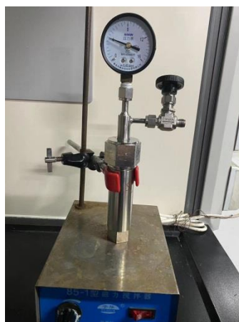
Figure S1 The setup for the synthesis of gem-dicarboxylic esters
