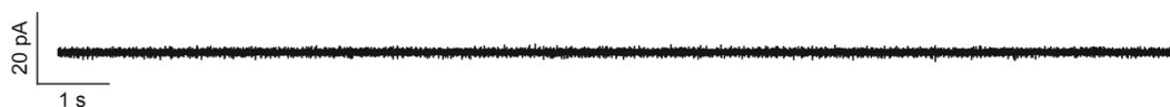
Fig. S10 Representative amperometric traces recorded after the insertion of a SiC@C NWE into macrophages after 24 h phagocytosis at +800 mV.
