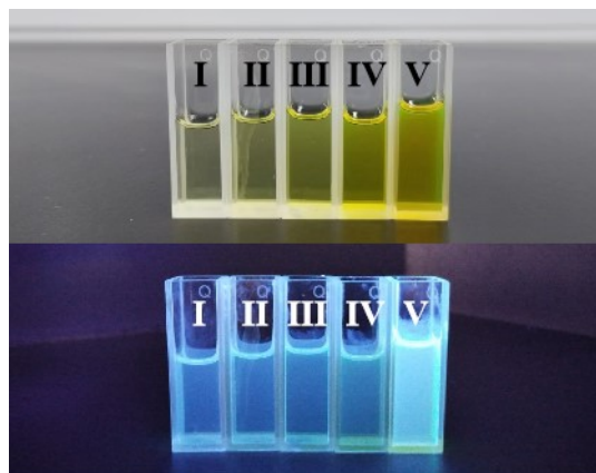
Fig S8. PL Intensity of CQDs dispersed in water at different concentrations: C_I=6.25\% ; C_{II}=12.5\% ; C_{III}=25\% ; C_{IV}=50\% ; C_V=100\% .
