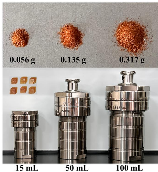
Figure S5. The scale-up synthesis of \text{Fe}_7\text{Sn}_6 .
