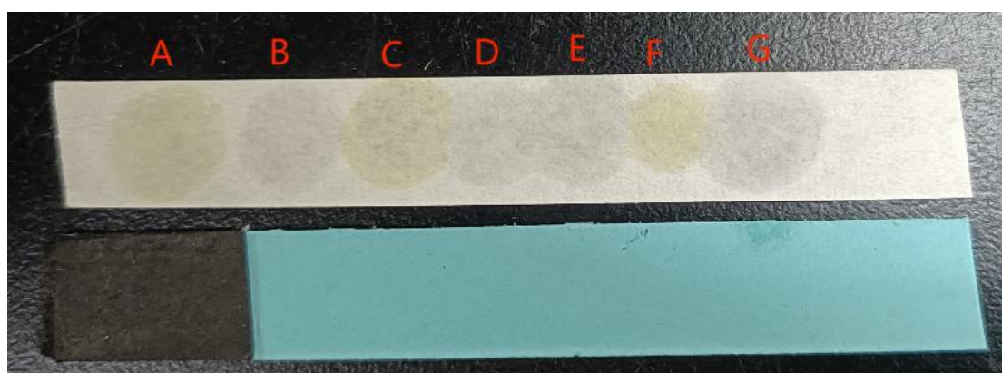
Figure S5. Bromine detected with starch potassium iodide test paper
