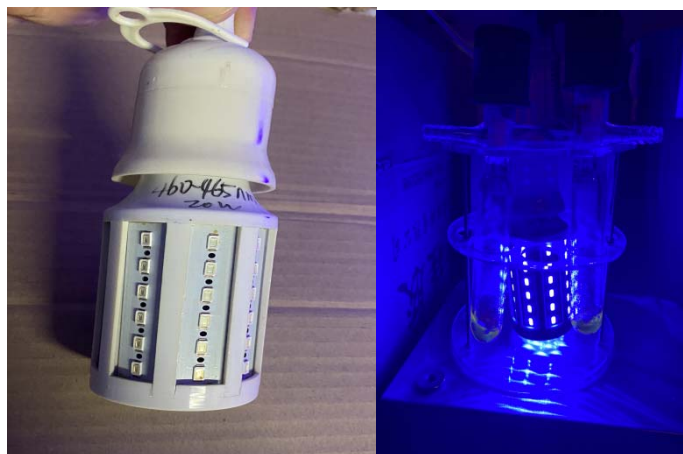
Figure S1. Photoreactor used in this work (20 W blue LEDs, \lambda_{\text{max}} = 465 nm).
