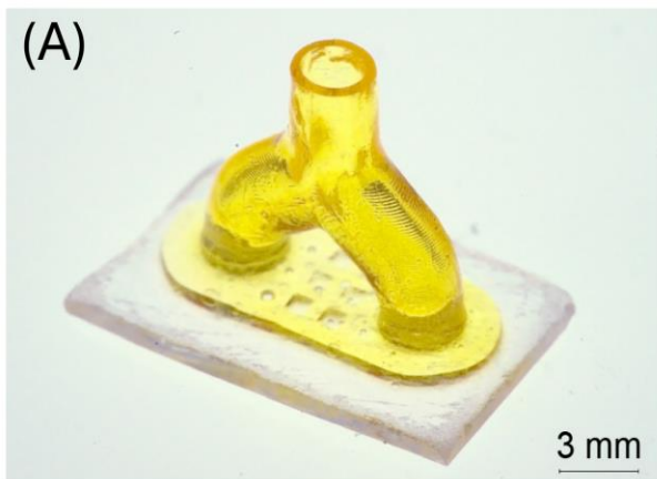
Figure S25. (A/B) Photographs of a blood vessel print, which was prepared using 20 mW/cm 2 405 nm LED, 12 s/100 μm layer, and 4 base layers at 20 s/100 μm layer. Outer diameter = 3 mm, inner diameter = 2.3 mm.
