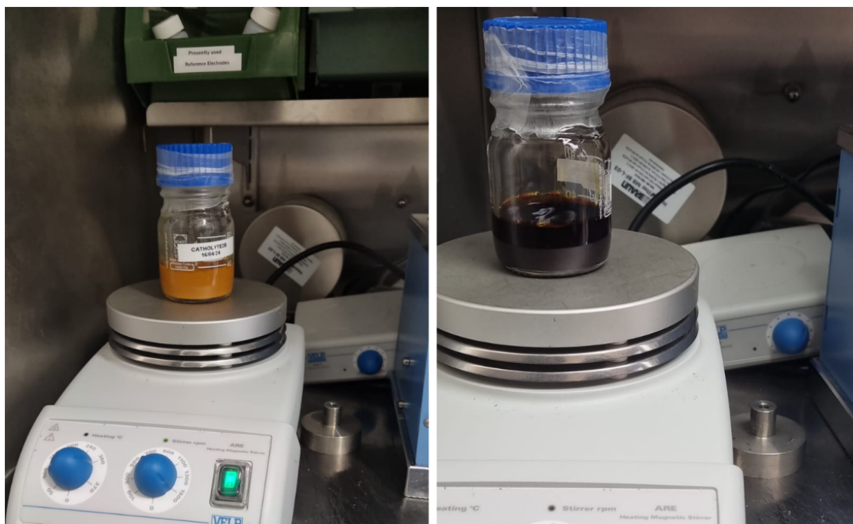
Figure S1. Photographic images taken upon the catholyte preparation. Left panel shows the first stage of the process, right panel displays the precursor after 7 h stirring at 70 °C and 48 h stirring at room temperature just before salts addition.
