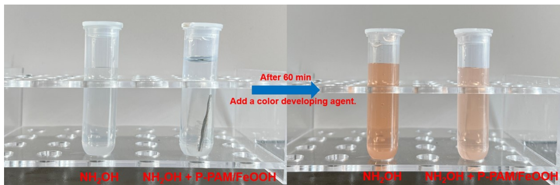
Fig. 21. Illustration of the experimental results for the adsorption of \text{NH}_2\text{OH} by P-PAM. The results indicate that after placing the working electrode P-PAM/FeOOH in the \text{NH}_2\text{OH} solution, the concentration of \text{NH}_2\text{OH} in the solution decreased (the lighter the color, the lower the concentration of \text{NH}_2\text{OH} ). This demonstrates that P-PAM has an adsorption effect on \text{NH}_2\text{OH} .
