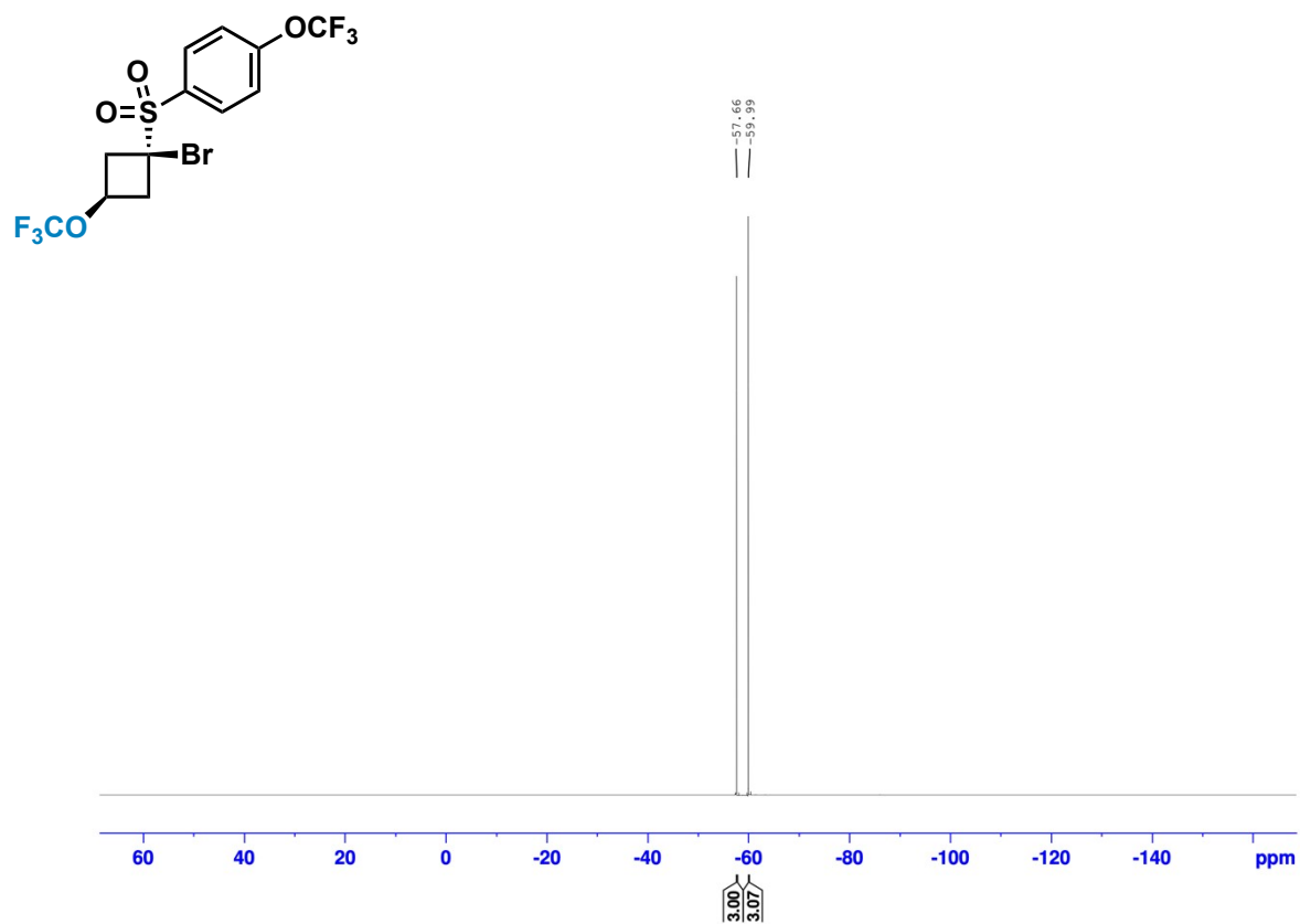
Figure S22. ^{19}\text{F} NMR spectrum of 1-((1-bromo-3-(trifluoromethoxy)cyclobutyl)sulfonyl)-4-(trifluoromethoxy)benzene (compound 4, syn isomer) in \text{CDCl}_3 .
