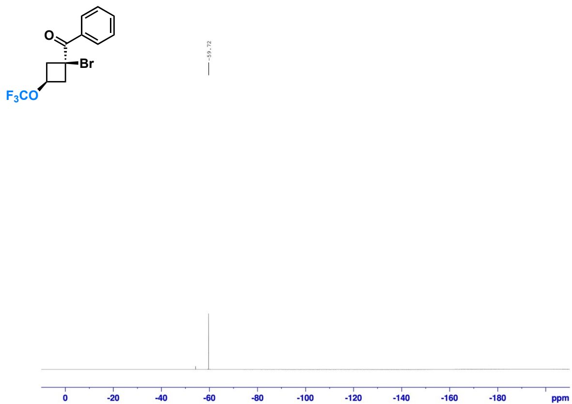
Figure S49. ^{19}\text{F} NMR spectrum of (1-bromo-3-(trifluoromethoxy)cyclobutyl)(phenyl)methanone (compound 12 , syn isomer) in \text{CDCl}_3 .
