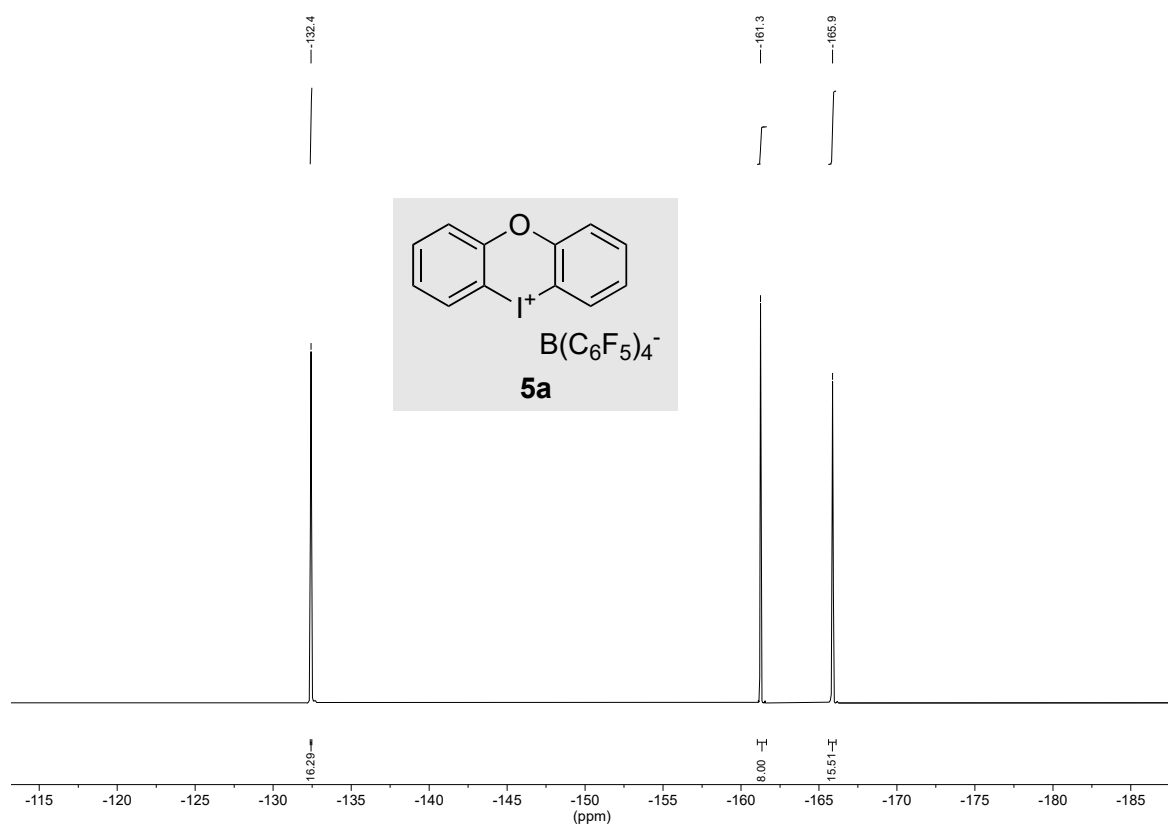
Figure S14. 565 MHz ^{19}\text{F} -NMR spectrum of compound 5a in \text{DMSO-}d_6 .
