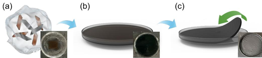
Fig. S7 Reusable operations of the film: (a) mixing the wasted film, (b-c) transferring and dissolution.
