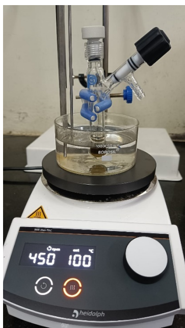
Figure S3. Reaction set up for the C–C coupling between 1a (0.5 mmol) and toluene (10 eq, 0.5 mL) at 100 °C using screw cap schlenk tube
