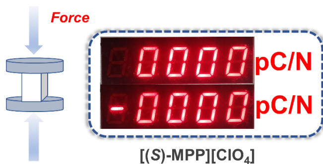
Fig. S8. The longitudinal piezoelectric coefficient value of [(S)-MPP][ClO 4 ].
