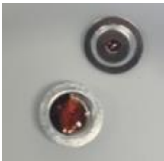
Figure S 38 Image of the orange liquid obtained (1-IL) from heating 1·3H 2 O to 150 °C.
