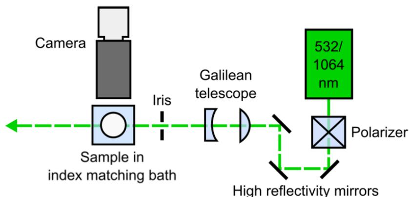
**Fig. S2.** A schematic diagram showing a typical optical setup for the irradiation of samples, including a polarizer (used for adjusting the laser power) and a Galilean telescope and iris (used for adjusting the beam diameter).
