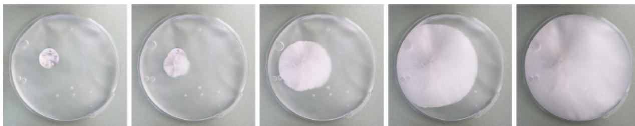
**Fig. S1.** Images of a reusable handwarmer, containing supersaturated aqueous sodium acetate solution, crystallising after the metal disk within is flexed. The formation of sodium acetate trihydrate crystals is rapid (approximately 10 s) and results in the release of heat.
