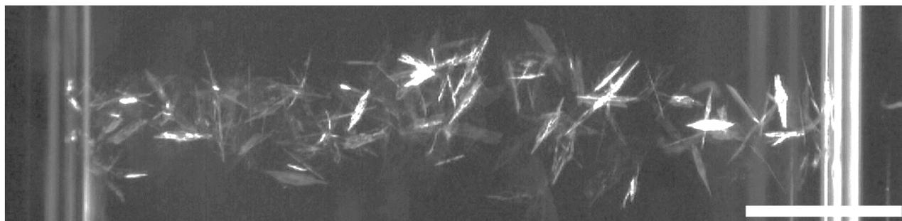
**Fig. S3.** Close-up of plate-like sodium acetate crystals following NPLIN with a single laser pulse growing in a supersaturated aqueous solution ( $C = 16.7 \text{ mol kg}^{-1}$ ,  $S = 2.72$ ) with no Na-PMAA polymer additive. The incident laser pulse had an energy density of  $27.6 \text{ mJ cm}^{-2}$ . The image was taken 87 s after exposure to the laser pulse, before the emergence of cloud-like crystals. Scale bar represents 2 mm.
