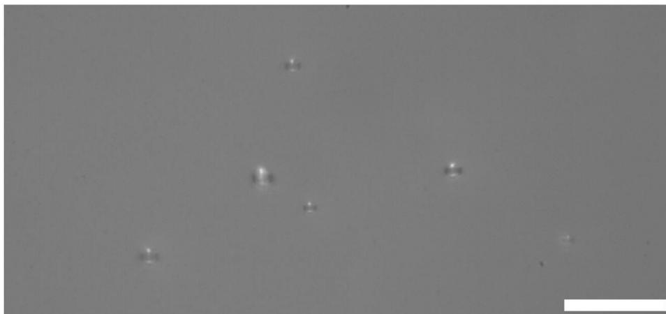
**Fig. S4.** Image of bubbles in a supersaturated aqueous solution of sodium acetate ( $C = 16.7 \text{ mol kg}^{-1}$ ,  $S = 2.72$ ) containing high Na-PMAA (0.73% w/w), following exposure to a single laser pulse. The incident pulse had an energy density of  $221 \text{ mJ cm}^{-2}$ . The image was taken approximately 13 minutes after the laser pulse. Bubbles are clearly identifiable, and a range of bubble sizes is observed. Scale bar represents  $100 \mu\text{m}$ .
