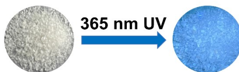
Fig. S9. Images of compound 2 crystals under natural light (left) and 365 nm UV light excitation (right).
