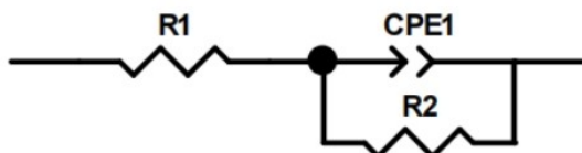
Fig. S9. OER-EIS fitting data for Ni 3 S 2 -Fe-Ni
