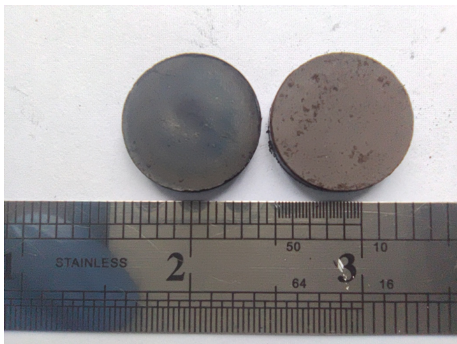
Fig. S1 Image of synthesized MnB(left) and precursor(right) block. The unit of the ruler is 1 inch.
