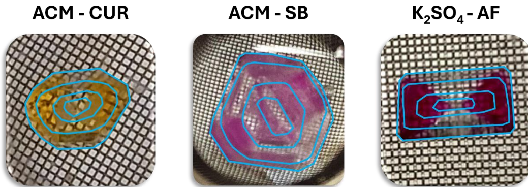
Fig. S4 Overlay of the crystal morphology changes during the dissolution experiments. For ACM-CUR, lines represent the state of the crystal after 2 min, 30 min, 55 min, and 64 min. For ACM-SB, lines represent the state of the crystal after 0 h, 1 h, 3 h, and 5.5 h. For K_2SO_4 -AF, lines represent the state of the crystal after 0 min, 5 min, 13 min, and 17 min.
