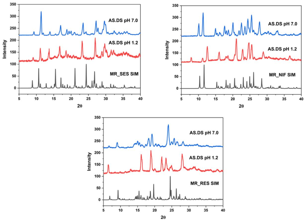
**Figure S5:** PXRD data of all molecular adducts after dissolution in both pH 1.2 and pH 7.0 indicated that MR.SES was stable, whereas MR.NIF and MR.RES partially transformed to either NIF or RES.
