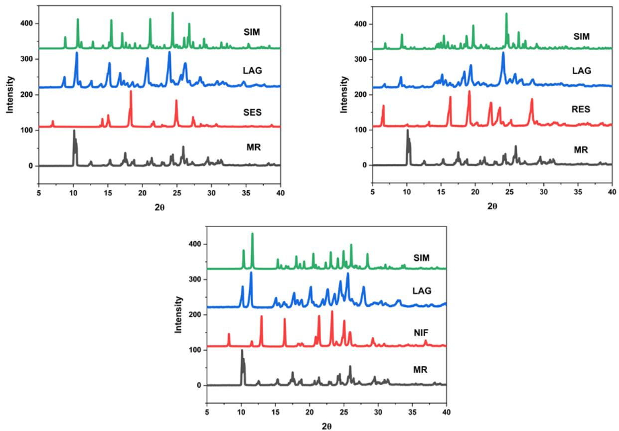
**Figure S2.** PXRD of all synthesized MR.SES, MR.NIF and MR.RES cocrystals confirmed their utmost purity.
