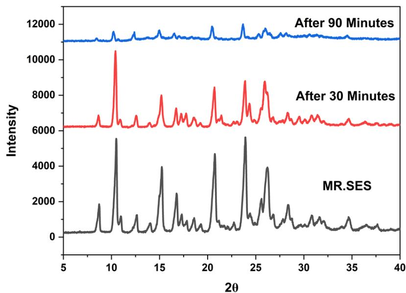
**Figure S6:** Time-dependent PXRD plot of MR.SES during solubility studies at pH 7.0, illustrating structural stability and decrease of particle size over time.
