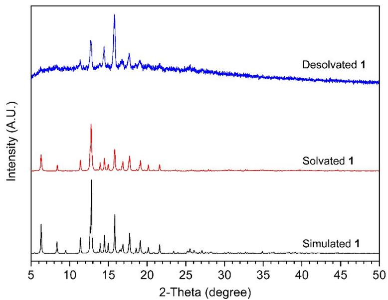
**Fig. S1** Comparison of the simulated, 1 and desolvated PXRD patterns for **SOF-1**.
