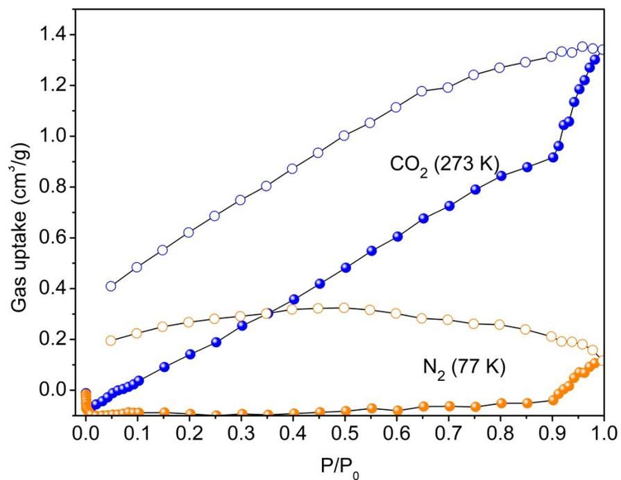
**Fig. S3** N<sub>2</sub> (77 K) and CO<sub>2</sub> (273 K) adsorption isotherms of SOF-1.
