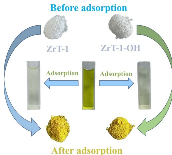
Fig.S6 Color change of TAR solution and Zr-MOCs before and after adsorption.
