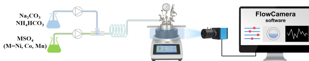
Fig. S1. Schematic of set-up for the synthesis of Ni-based carbonate materials.
