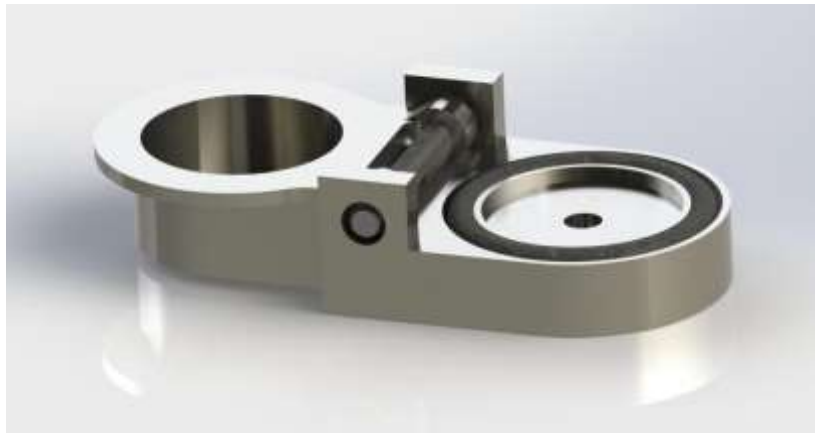
Figure S7. Vacuum transfer chamber for electron microscope. The sample is mounted inside the chamber in a glovebox, then chamber is closed and evacuated in antechamber of a glovebox. Atmospheric pressure secures the chamber shut, while a pre- tensioned spring releases the cap in the SEM chamber once vacuum equilibrium is achieved.
