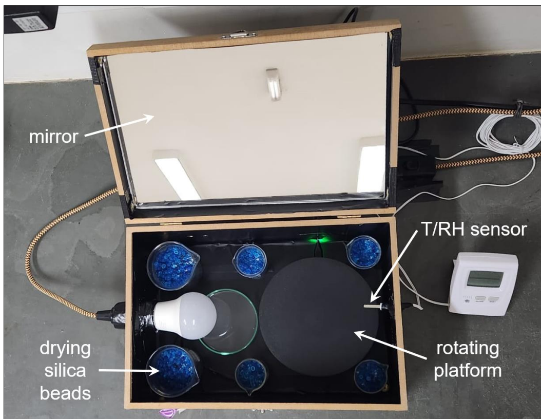
Figure S1 - Homemade setup used for the light-accelerated degradation test. The samples were distributed uniformly in the Petri dish, which was positioned in the center of the rotating (6 Hz clockwise) platform and submitted to direct and mirror-reflected illumination from the LED lamp. The lamp specifications are a power of 6 W, luminous flux of 560 lm, and color cold white (6500 K). The box (30 x 20 x 15 cm) remained closed and sealed with masking tape during the test. Inside humidity was kept as low as possible by drying silica beads. Temperature and relative humidity were constantly monitored, ranging from 25 to 32 °C and 35 to 50 % throughout the experiment.
