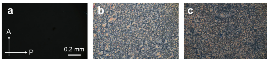
Figure S6. Textures of MB-PB-22 at (a) 432.9 K (Cub), (b) 368.3 K ( Cr_4 ), and (c) 324.3 K ( Cr_1 ) on cooling ( 5 \text{ K min}^{-1} ).
