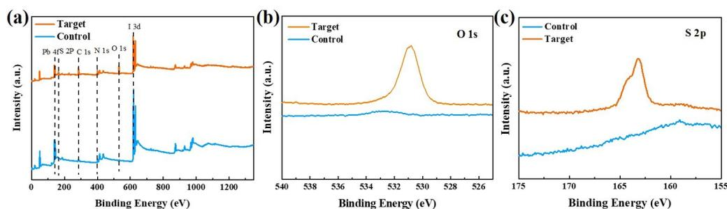
**Figure S6.** (a) XPS spectra of control and target perovskite films; XPS spectra of (b) O 1s and (c) S 2p in control and target perovskite films.
