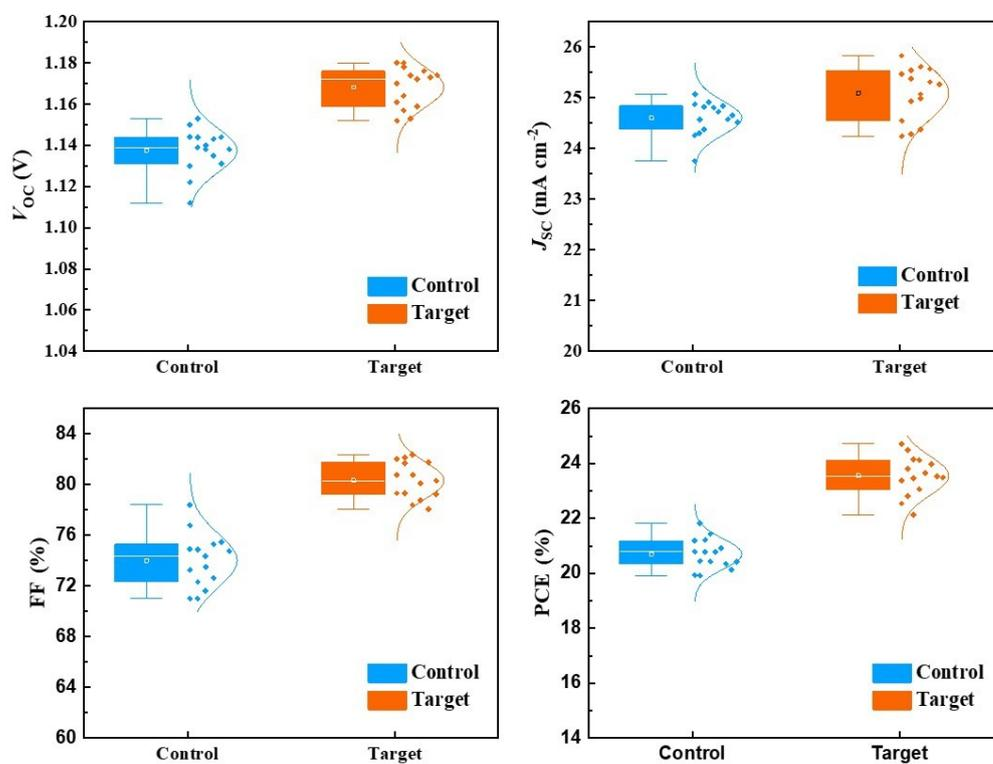
**Figure S2.**  $V_{OC}$ ,  $J_{SC}$ , FF, and PCE distribution of 15 individual control and target PSCs.
