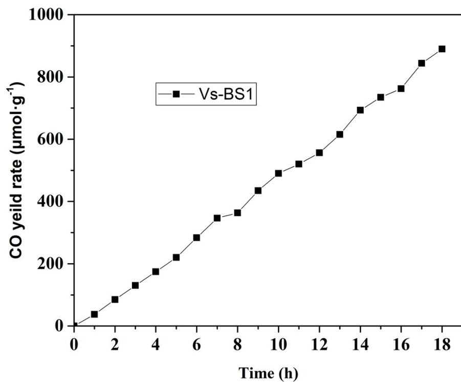
**Fig. S4** The stability of photocatalytic performance of Vs-BS1 under the irradiation of a 300 W xenon lamp after 18 hours.
