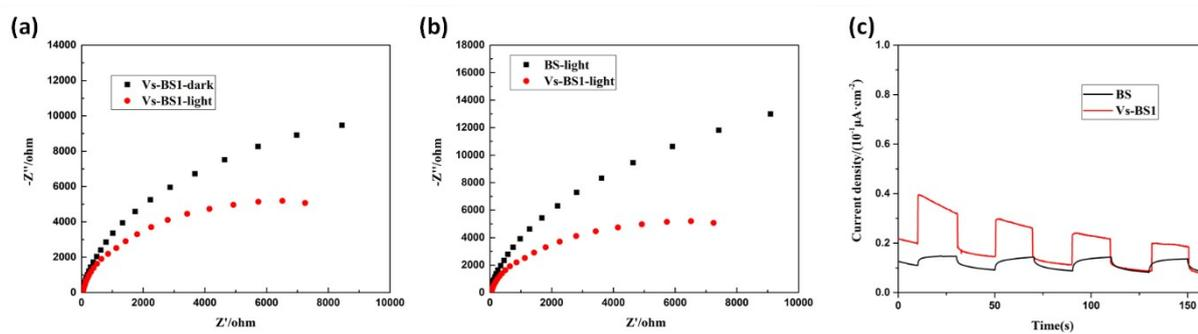
**Fig. S2** (a) EIS Nyquist plots of the Vs-BS1 in the light and in the dark (b) EIS Nyquist plots of the BS and Vs-BS1 in the light (c) Transient photocurrent responses of BS and Vs-BS1.
