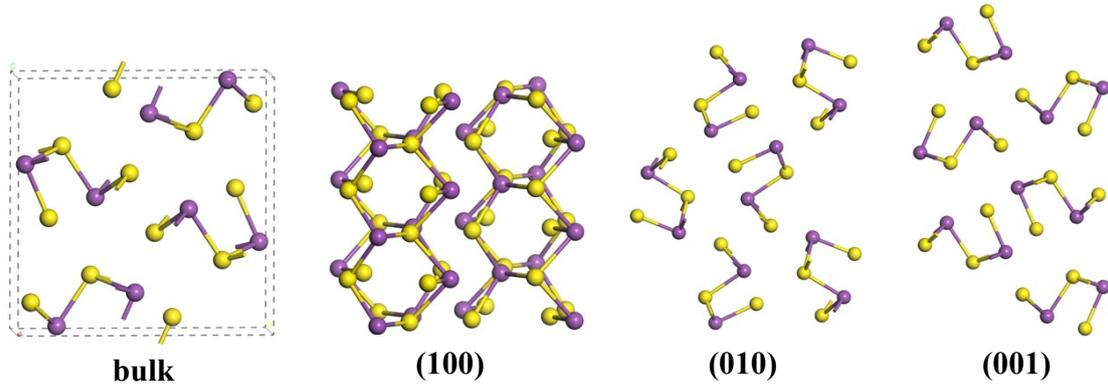
**Fig. S5** Illustration of bulk and low-indexed surfaces of  $\text{Bi}_2\text{S}_3$ . The purple and yellow balls represent Bi and S atoms, respectively.
