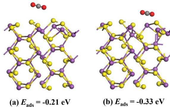
**Fig. S6** The optimized structures and the calculated adsorption energies of a  $\text{CO}_2$  molecule supported on (a) the clean surface and (b) the surface with a S vacancy in the top layer.
