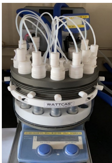
118 Fig. S5. The photocatalytic reactions were performed by a photoreactor from WATTCAS WP- 119 TEC-1020HS
