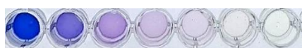
Figure S8. Colorimetric assay calibration of 2a in KPi buffer (50 mM, pH 7.5)
