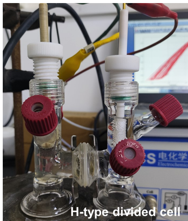
Figure S3. Digital photograph of H-type divided cell reactors.
