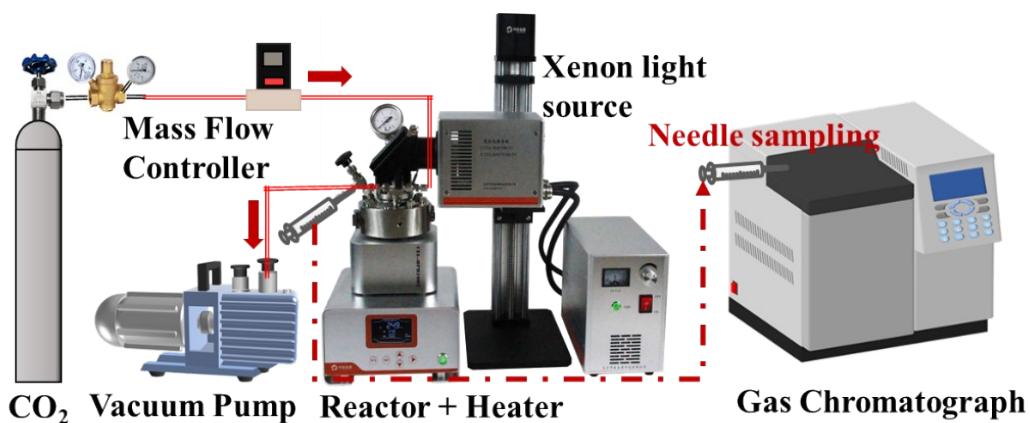
Figure S3 Schematic diagram of the photothermal coupling catalyst performance evaluation system test
