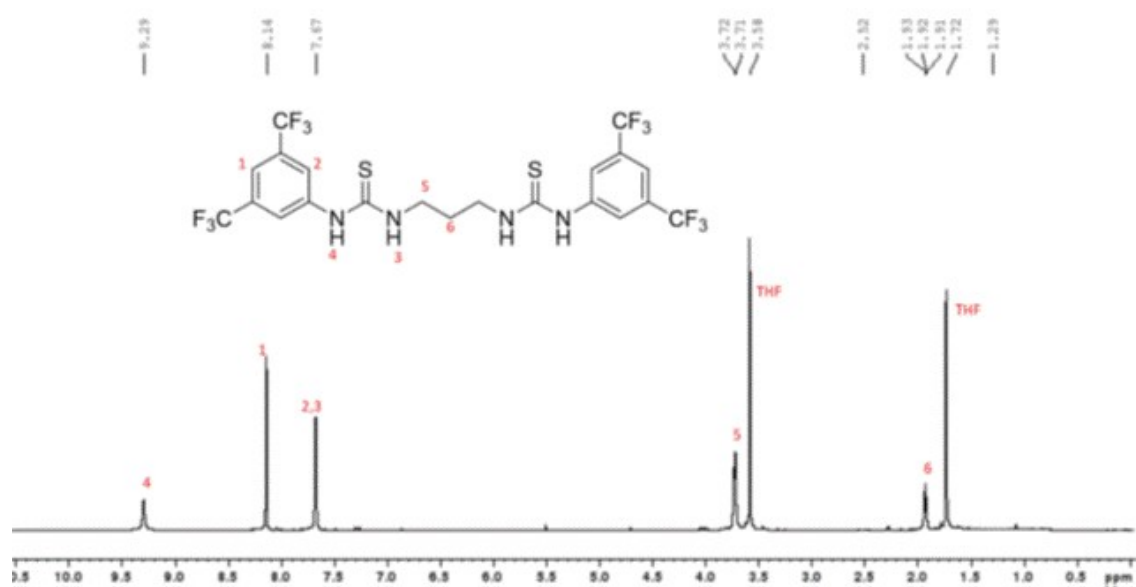
Figure S2. 1 H NMR spectrum (400 MHz, THF d 8 , 298 K) of the bis(thio)urea TU
