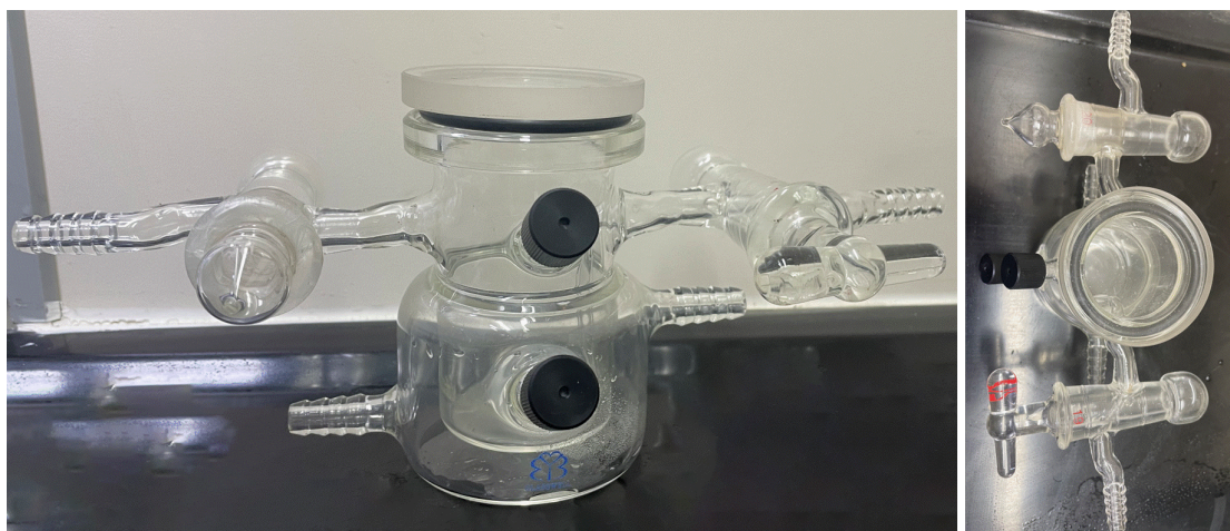
Figure S34. Photo-reaction vessel with radius 2.25 cm. The radius of stir bar is 0.5 cm.
