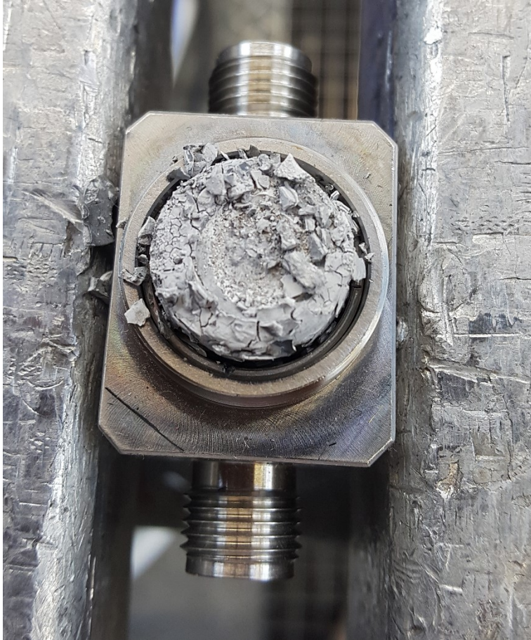
Figure 8: Clogged filter with precipitated TINUVIN 770 (taken from pre-experiments).
