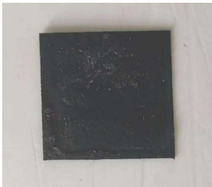
Figure S13. GDE after 10h reaction in 1M KOH (carbonate formation on the surface)
