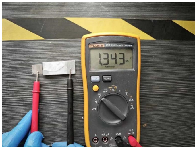
Fig S12. Photograph of flexible RZAB of Pt/C+Ru/C cathode with an open-circuit voltage of 1.343 V.
