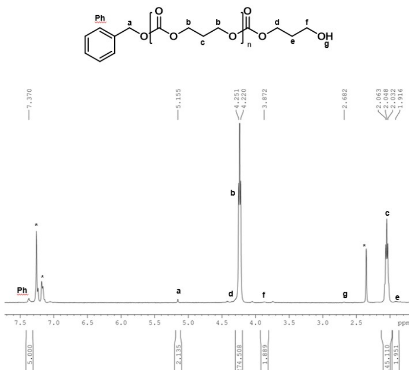
Figure S17: ^1\text{H-NMR} spectrum of poly(trimethylene carbonate) (solvent: \text{CDCl}_3 , 400 MHz, 298 K). * = toluene.
