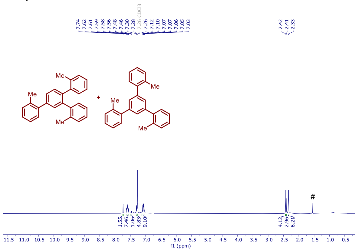
^1\text{H} NMR of 2,2''-dimethyl-4'-(o-tolyl)-1,1':2',1''-terphenyl (Compound 3l) in \text{CDCl}_3 . # indicates the solvent impurity of \text{H}_2\text{O} in \text{CDCl}_3 .
