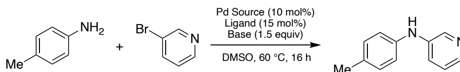
Figure S3. General reaction scheme for the Buchwald-Hartwig coupling.
