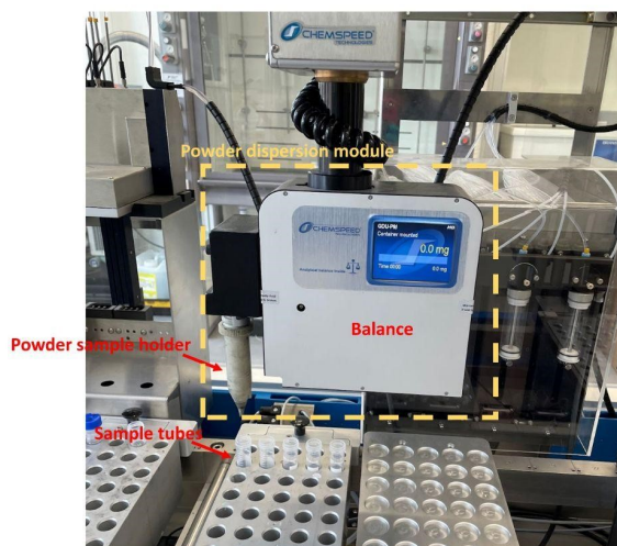
Figure S12. Image of the powder dispensing module within the Chemspeed system.
