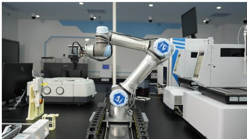
**Supplementary Fig. S11. Benchtop robot.** The benchtop robot is used to flexibly clamp and transfer samples on an integrated clamping, separation and measurement operations.
