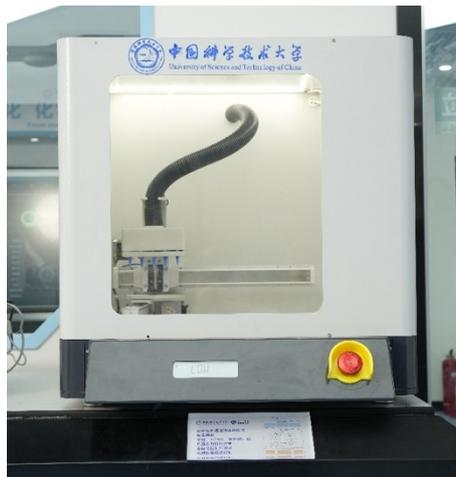
**Supplementary Fig. S15. Liquid station.** The liquid station is used to add pre-configured liquid reagents (ten different reagents can be placed at the same time). Parameters that can be set are mass (g) and the type of liquid.
