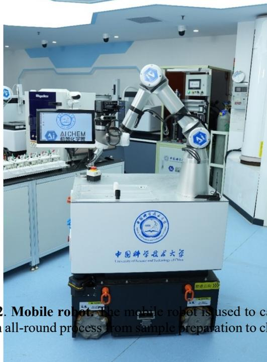
**Supplementary Fig. S12. Mobile robot.** The mobile robot is used to carry and transport samples in an automated lab for an all-round process from sample preparation to characterization and testing.
