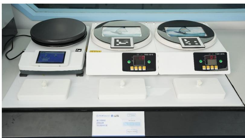
**Supplementary Fig. S17. Magnetic stirring station.** The magnetic stirring station is used to mix and stir different reagents (heating permitted) to obtain homogeneous solutions or sample dispersions. Parameters that can be set are time (s), temperature ( $^{\circ}\text{C}$ ) and angular velocity (rpm).
