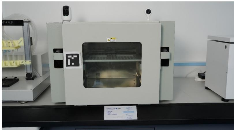
**Supplementary Fig. S21. Drying station.** The drying station is used to dry samples. Parameters that can be set are time (s) and temperature (°C).
