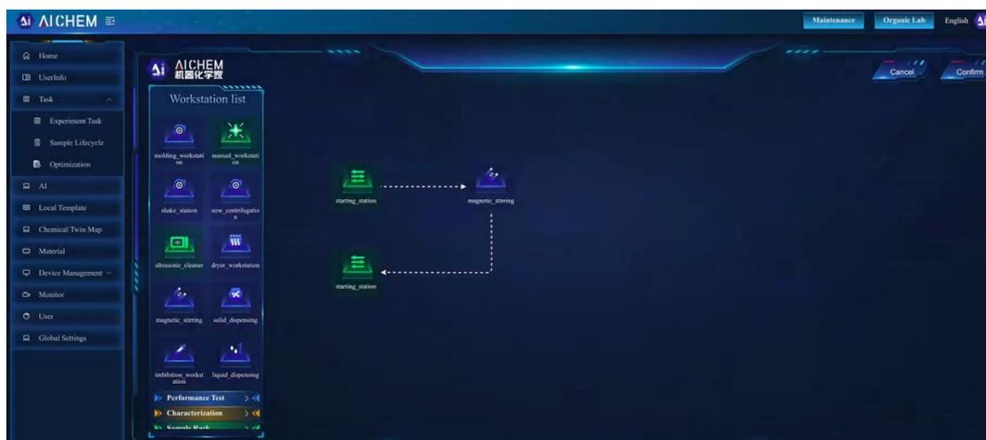
**Supplementary Fig. S28. The interface for users to assign experiments.** Users can select components from the left panel, drag them into the central area to connect and form a task flow, and confirm the assignment in the top-right corner.
