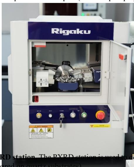
**Supplementary Fig. S26. PXRD station.** The PXRD station is used to determine the phase composition of samples (with samples prepared on quartz substrates).
