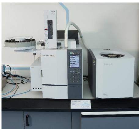
**Supplementary Fig. S24. Gas chromatography station.** The gas chromatography station is used to measure the gas production of reaction systems.
