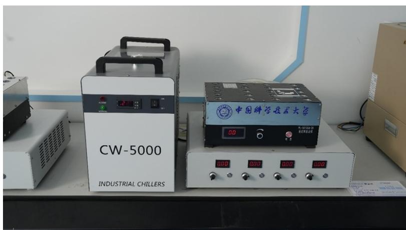
**Supplementary Fig. S23. Photocatalytic station.** The photocatalytic station is used to carry out light irradiation with simultaneous agitation. The parameter that can be set is the time (s).
