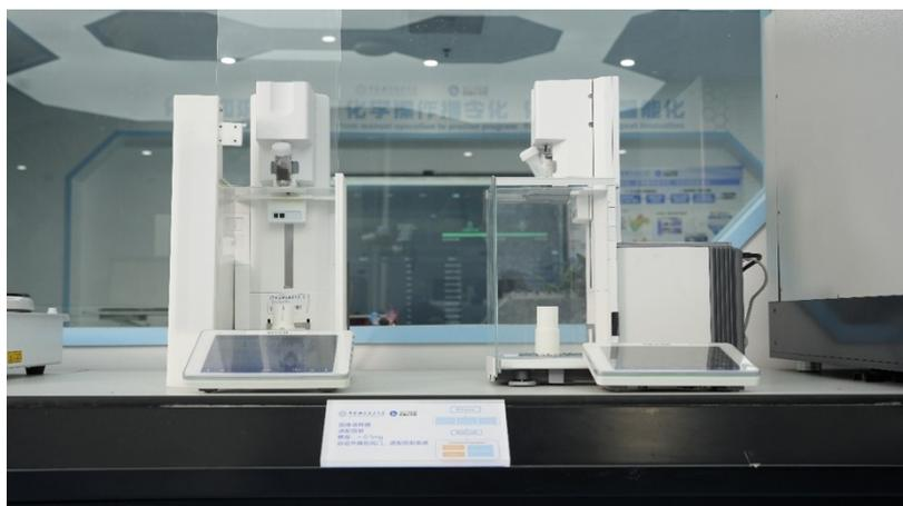
**Supplementary Fig. S16. Solid station.** The solid station is used to add pre-filled solid reagents. Parameters that can be set are mass (g) and the type of solid.
