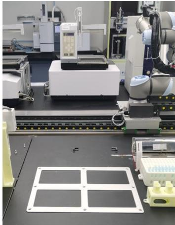
**Supplementary Fig. S14. Multi-robot exchange station.** The multi-robot exchange station is used for transferring samples between the high-throughput platform and other experimental stations in the laboratory.
