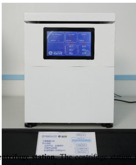
**Supplementary Fig. S18. Centrifuge station.** The centrifuge station is used to separate mixtures of liquids and solid particles. Parameters that can be set are time (s) and angular velocity (rpm).
