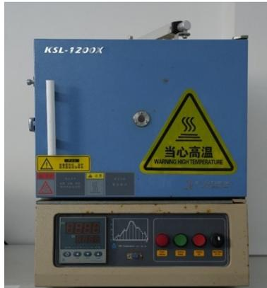
**Supplementary Fig. S19. Calcination station.** The calcination station is used to calcine and heat samples. Parameters that can be set are time (s) and temperature (°C) and heating rate (°C/min).
