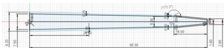
Opentrons 1000  $\mu\text{L}$  pipette tip (reproduced from <https://www.genfollower.com/1000ul-pipette-tip-for-opentrons/>):
