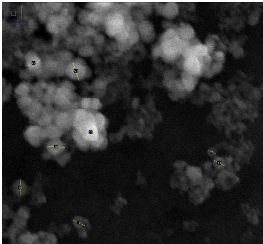
Figure S3. Magnified inset of micrograph from Figure S2 to highlight a sampling of particle diameter line selections in ImageJ software.
