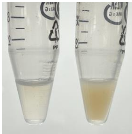
Figure S7. Comparison of relatively dilute (left) and relatively concentrated (right) Ce particle suspensions.
