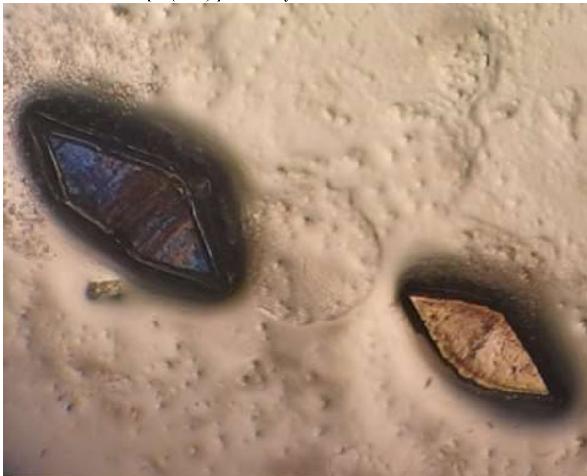
Figure S 3: Pictures of \text{Cs}_3[\text{Eu}(\text{DPA})_3] \cdot 9\text{H}_2\text{O} made following the description in the experimental section. The crystals have a difference in size, but all of the crystal were found to be clear, light, and colourless with a prism structure. All crystals were observed to have the same phase. The complex crystallises in the orthorhombic C222_1 space group.
