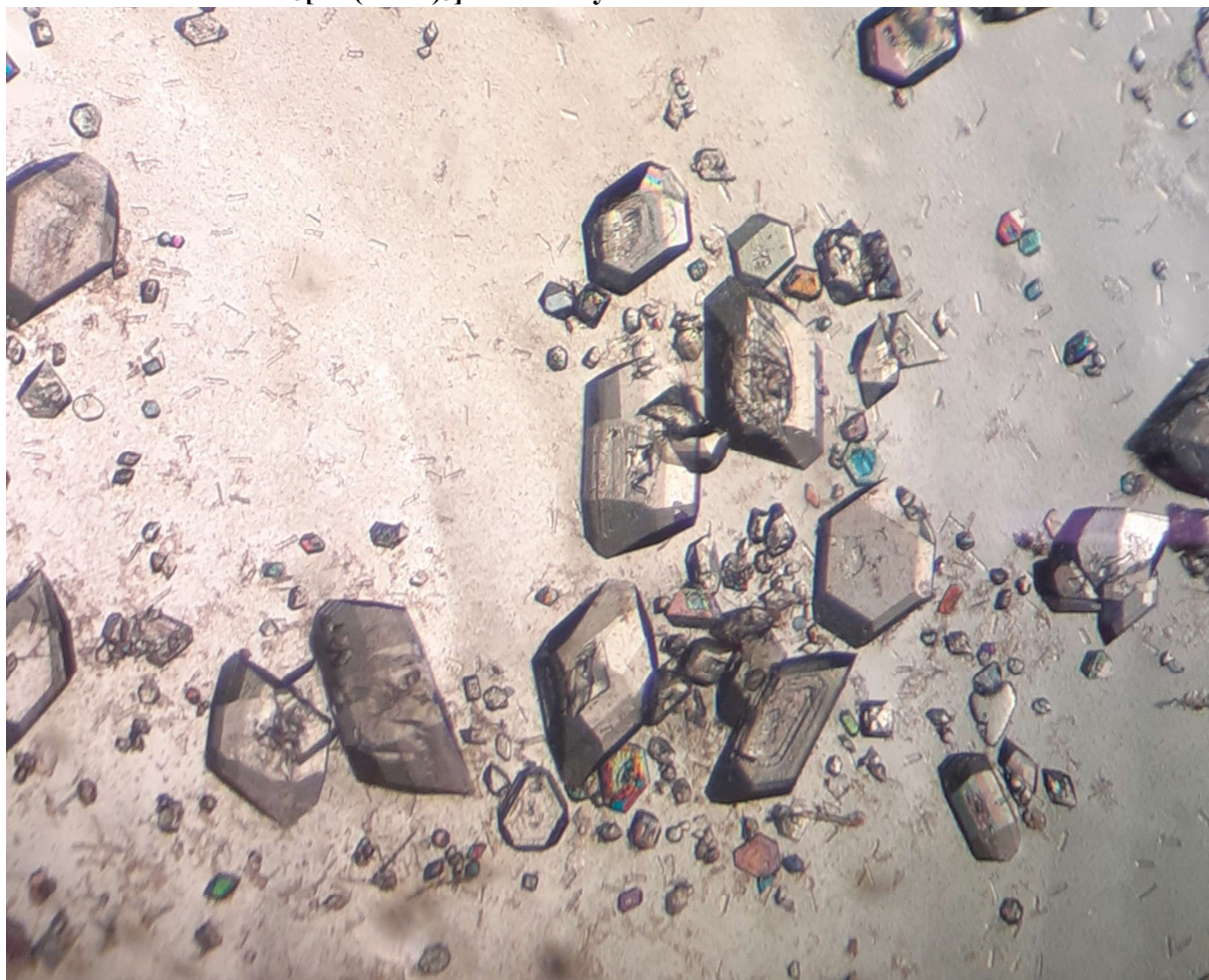
Figure S 1: Pictures of \text{Na}_3[\text{Eu}(\text{ODA})_3] \cdot 8\text{H}_2\text{O} made following the description in the experimental section. The crystals have a difference in size, but all of the crystal were found to be clear, light, and colourless with a prism structure. All crystals were observed to have the same phase. The complex crystallises in the monoclinic C2/c space group.
