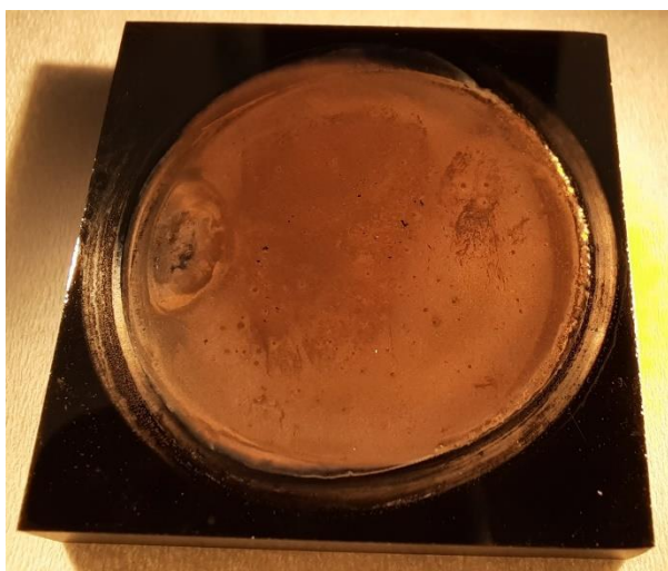
Figure S24. The larger GCWE ( A = 2.7 \text{ cm}^2 ) and cell setup at the start of the CPE (top) and after the CPE (bottom) using the large plate glassy carbon working electrode).
