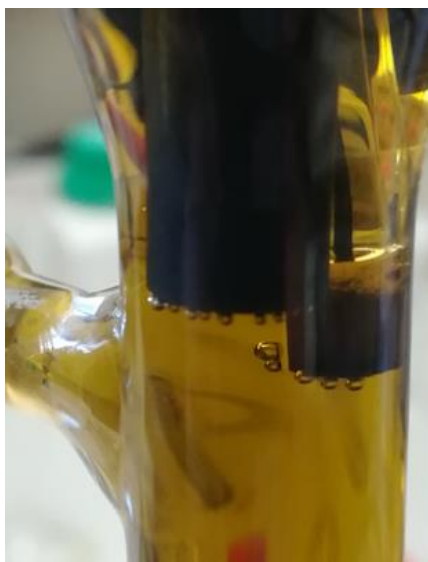
Figure S6. Visible evolution of bubbles on 3 mm glassy carbon working electrode ( A = 0.071 \text{ cm}^2 ) during recording the CPE of complex 1 in neutral aq. phosphate buffer. Conditions: 1 M pH 7 phosphate buffer solution, 3 mm glassy carbon working ( A = 0.071 \text{ cm}^2 ) and Pt counter electrode, Ag|AgCl reference, 100 mV/s.
