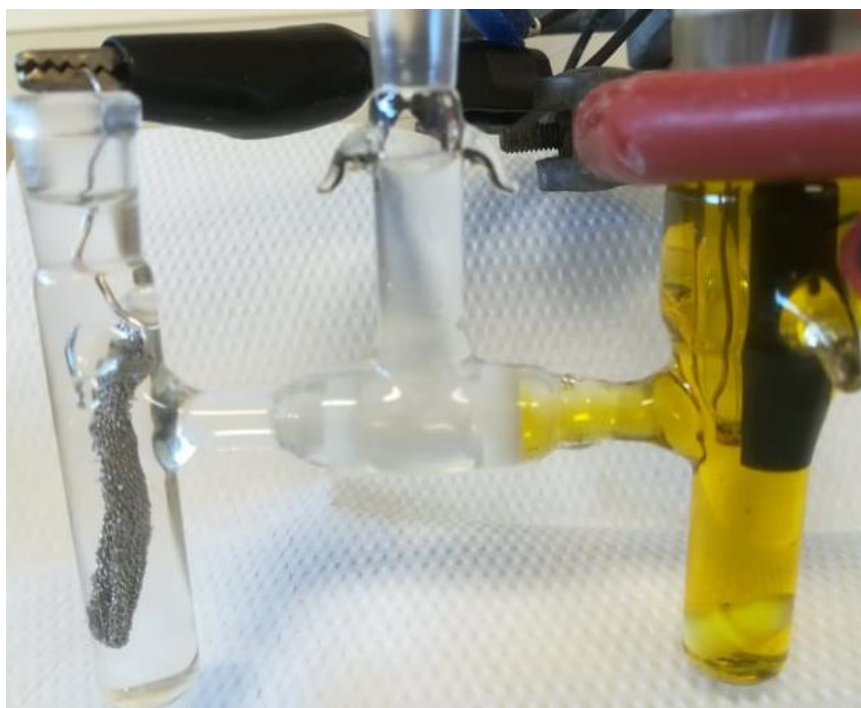
Figure S2. Example setup of small electrochemical “H-cell” used for cyclic voltammetry and some of the controlled potential electrolysis (CPE) experiments; other CPE experiments were carried out in a larger cell (see section S3 below). The right is the working chamber with [\text{Cu}^{\text{II}}\text{L}^{\text{Et}}]\text{BF}_4 (0.3 – 1 mM, usually 0.3 mM unless otherwise stated) present, the black rod is a small 3 mm diameter ( A = 0.071 \text{ cm}^2 ) glassy carbon working electrode (GCWE), and next to that is the reference electrode. The reference electrode is either 0.01 M \text{AgNO}_3|\text{Ag} or \text{Ag}|\text{AgCl} , used for the MeCN and aqueous experiments, respectively. The left side is the platinum counter electrode, either mesh (shown) or plate.
