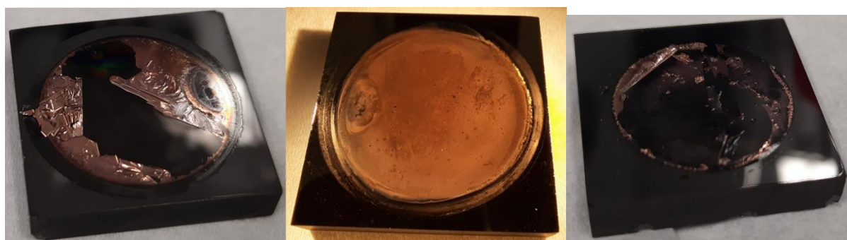
Figure S19. Cu(OAc) 2 ·H 2 O (left), [CuL Et ](BF 4 ) ( 1 ) (middle), and Cu(BF 4 ) 2 ·6H 2 O (right) deposits formed on the glassy carbon plate working electrodes after CPE at -1.1 V applied versus Ag|AgCl|sat. KCl, in 1M aq. phosphate buffer at pH 7.
