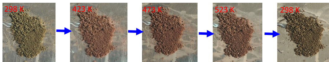
Figure S7. Variable-temperature images of 1-g , displaying the sequence of temperature changes following the direction of the arrow. 1-g is a poor conductor of heat, leading to non-uniform heating of its constituent particles. Consequently, certain particles in the sample back to 298 K attain higher temperatures than others, manifesting as a slight red hue in some powdered particles.
