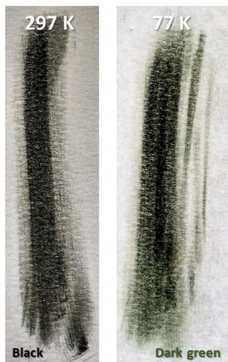
Figure S3. A reversible thermochromism from black T = 297 K to dark-green at T = 77 K (cooled with the liquid nitrogen).
